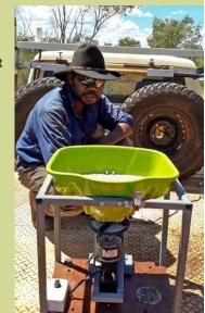
spreader from the driver's seat. The system uses the same power system rangers installed on the 100 litre quick-spray units issued with ATVs. Both units are designed for quick release and have common one-way electrical terminals to prevent cross-wiring.
