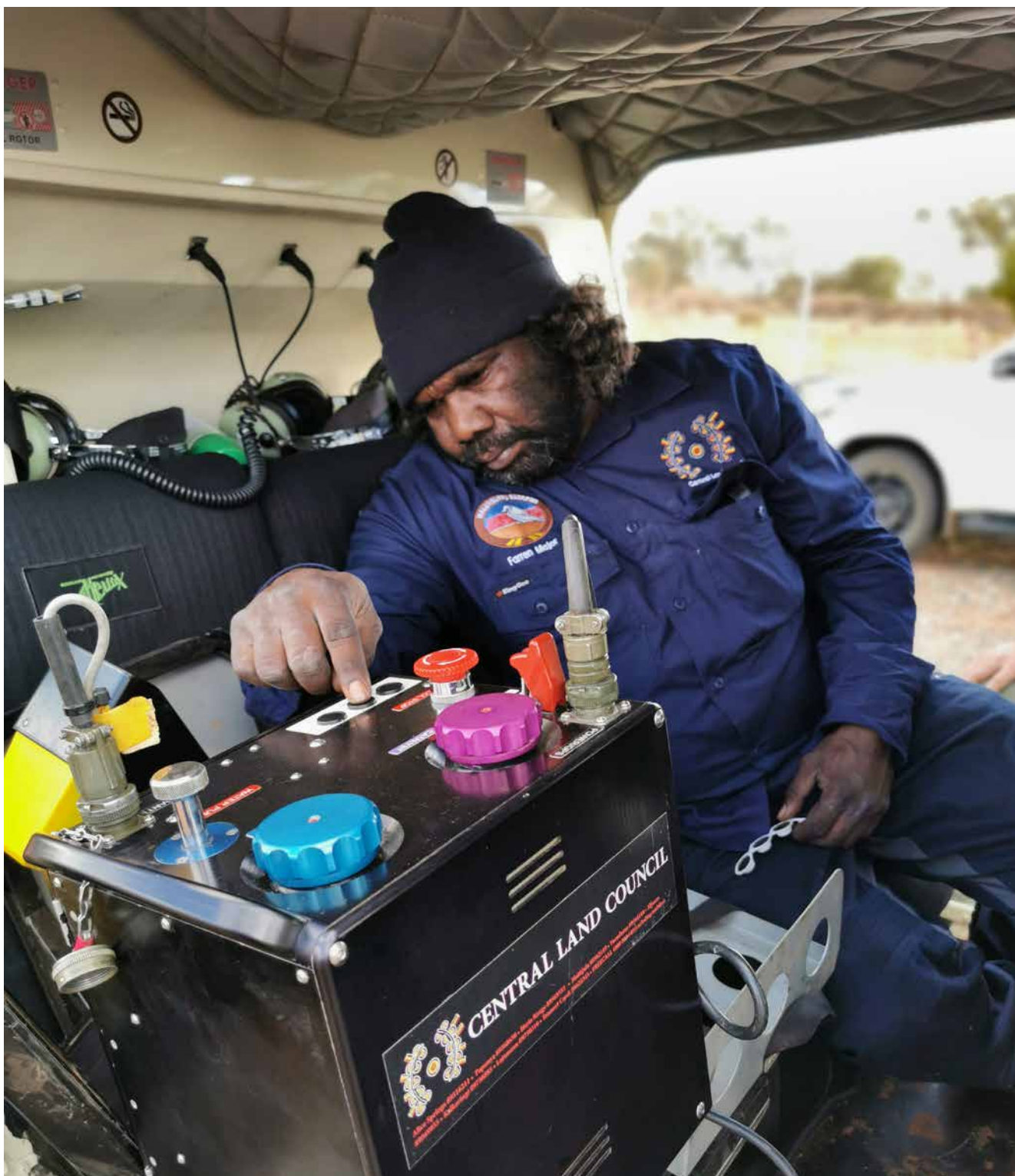
Farren Major checked the aerial incendiary device before conducting a helicopter burn.
