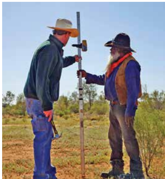
CLC ranger Gibson John (right) and the CSIRO's Ashley Sparrow use a laser level to mark erosion banks.
