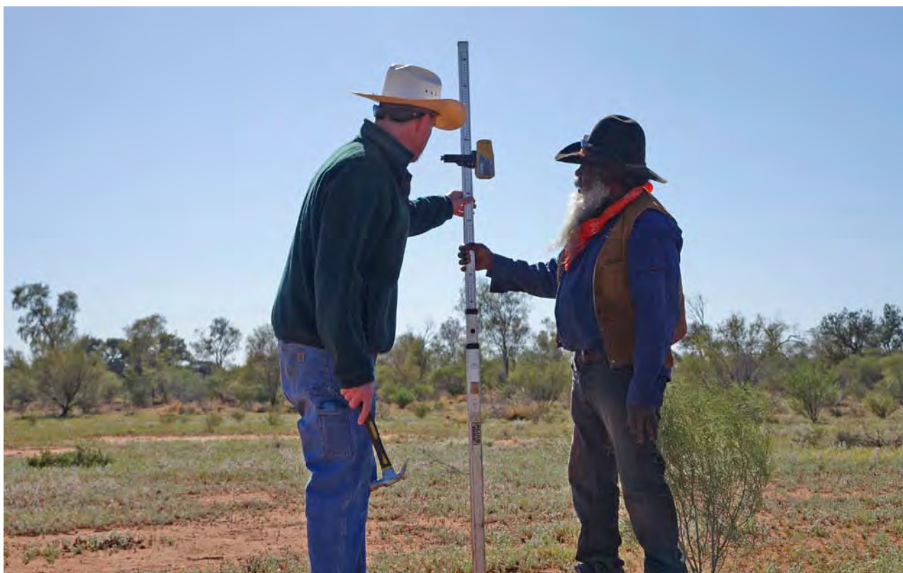
CLC ranger Gibson John (right) and the CSIRO's Ashley Sparrow use a laser level to mark erosion banks. Photo: Fiona Walsh, CSIRO.
